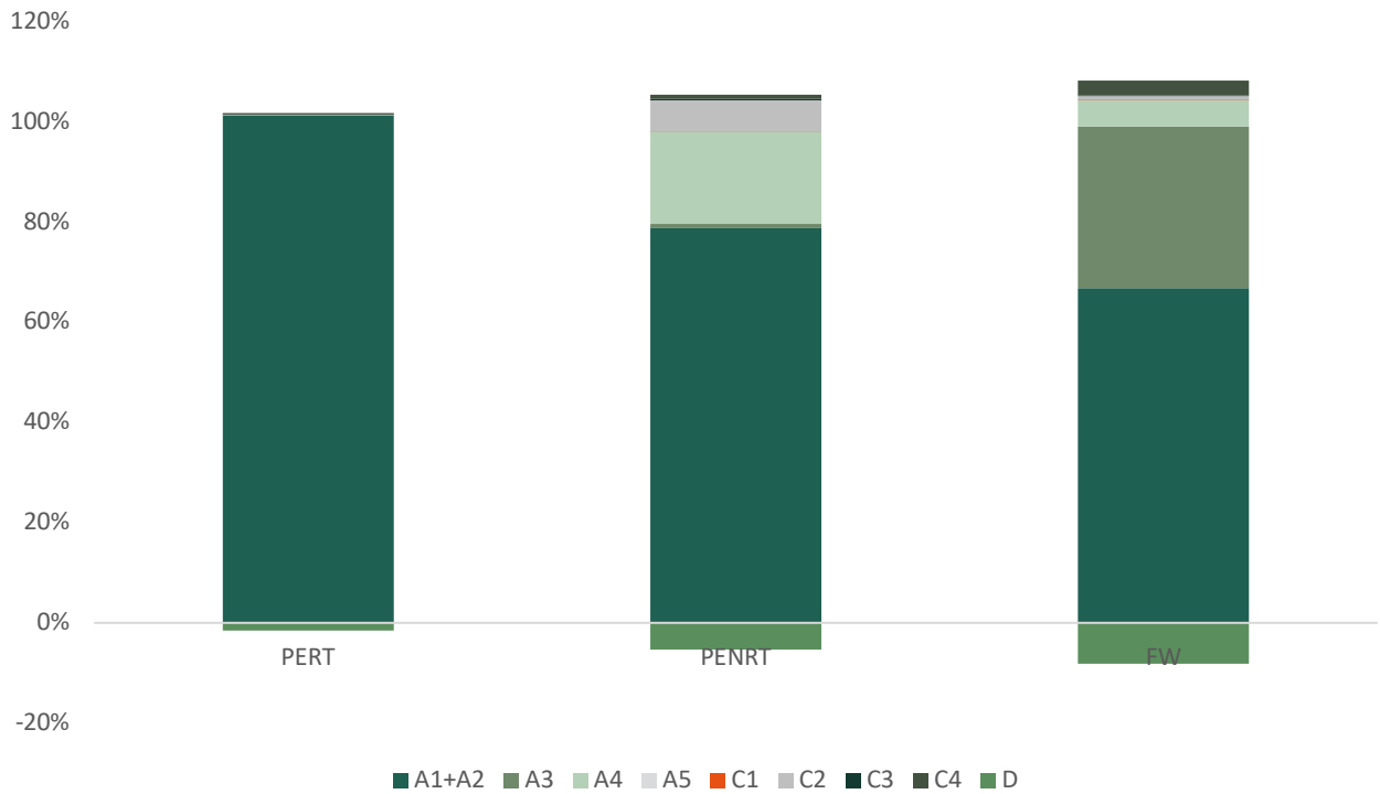
Figure 4 Percentage contribution of life cycle stages to the different resource use impact categories for the average plywood products manufactured by CMPC.
